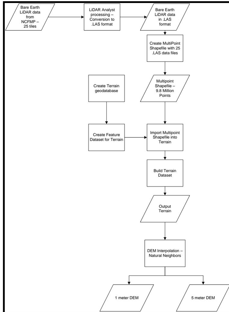
**Figure 3.** Flowchart of steps involved in creation of terrain dataset and digital terrain models from bare earth LiDAR data.
